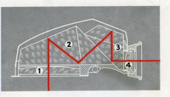
EYE-LEVEL PRISM FINDER FOR HASSELBLAD 500 C The viewfinder is comprised of a lens and prism system of very high optical quality. It provides an erect image about  $2\frac{1}{2}$  times the size of that appearing on the ground glass screen.
